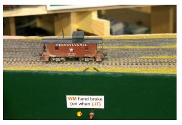
Did you ever want to stop a car on a grade (the pictured one is 2.1%) without having it roll back downhill? You can use a Tortoise switch machine to easily do this in only a few simple steps. You can even simply add an indicator LED. You will need access to the underneath side of the track — which should be in place and ballasted before starting to install your hill holder. Note that the location of the hill holder is marked with 2 ties in the photo.
