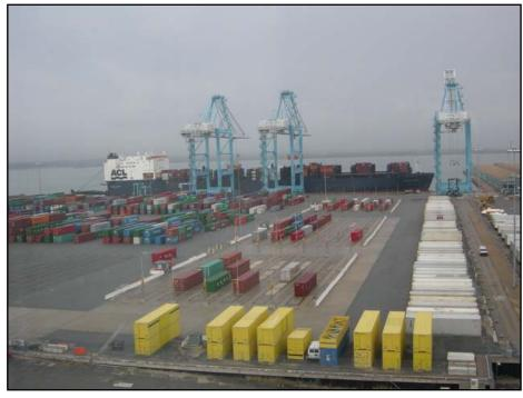
This view is facing east where we could see the entire yard. The yellow containers at the bottom of the photo are the port radiation detectors. The ACL ship at the dock was a standard 900 foot variety. The gantry cranes remove containers from the ship and place them on the dock next to the ship. Then straddle cranes pick the containers up for placement somewhere in the yard or directly on one of the trains being made up.
