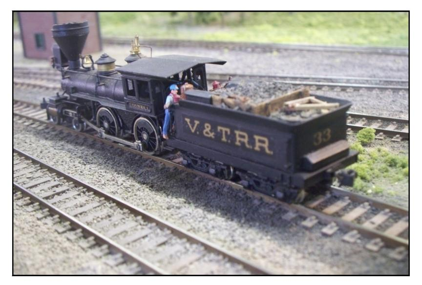
This picture is a locomotive which is a copy of V&TRR # 28 "Flanagan." It is a repainted and super detailed AHM Inyo modeled after the "Inyo" #22 of the V&TRR. The real #22 is currently preserved in the Southern California Railroad Museum. The original domes, bell, and stack were replaced with brass, and the back-head and cab were super detailed.
