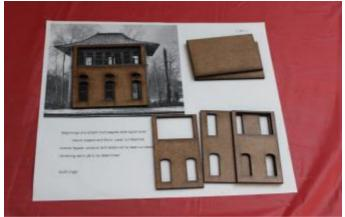
Scott Unger is scatchbuilding a DL&W pagoda-style tower. The walls are Masonite cut on a laser cutter.
