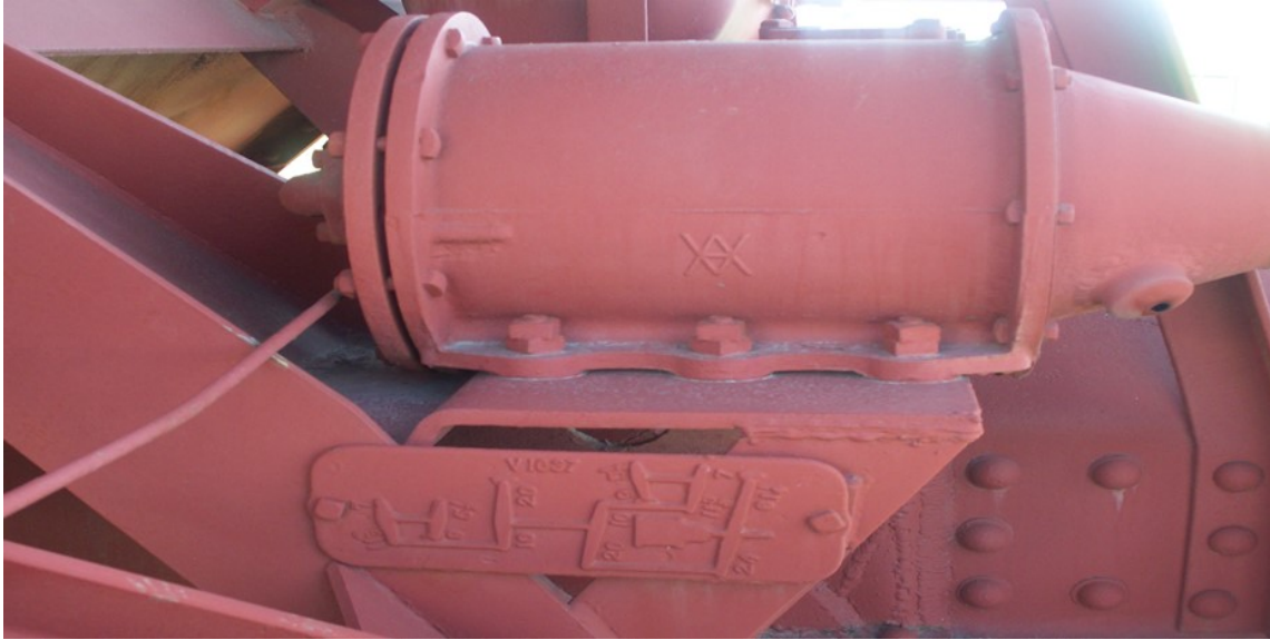
Right below the brake cylinder was a diagram of the cars brake system.
