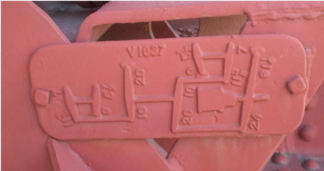
Right below the brake cylinder was a diagram of the cars brake system.
