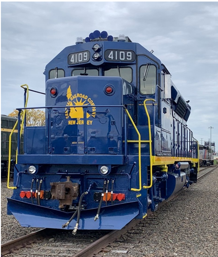
Currently used as a switcher, NJ Transit GP40H-2 No. 4109 will have HEP equipment installed for use on revenue trains.
