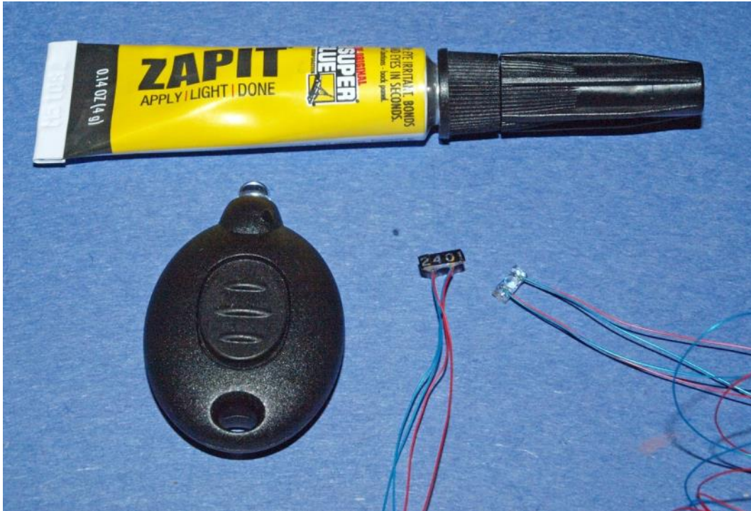
Glue the LEDs in place with ZAPIT
