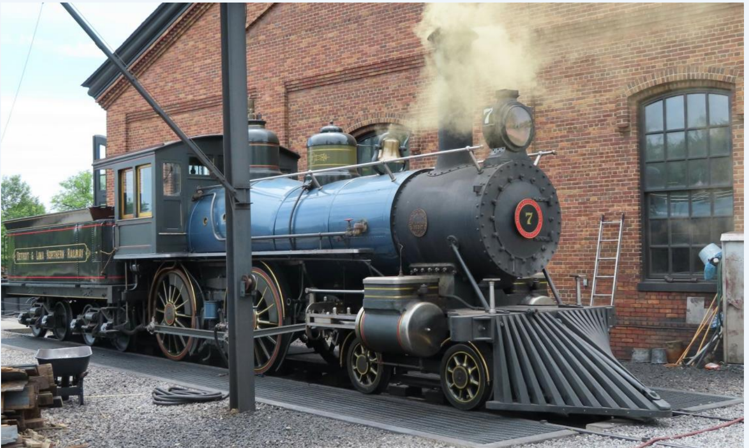
Baldwin-built engine #7 is a 4-4-0 locomotive owned by the Detroit & Lima Northern Railway. This restored engine is on display at the Greenfield Village, Dearborn, MI.
