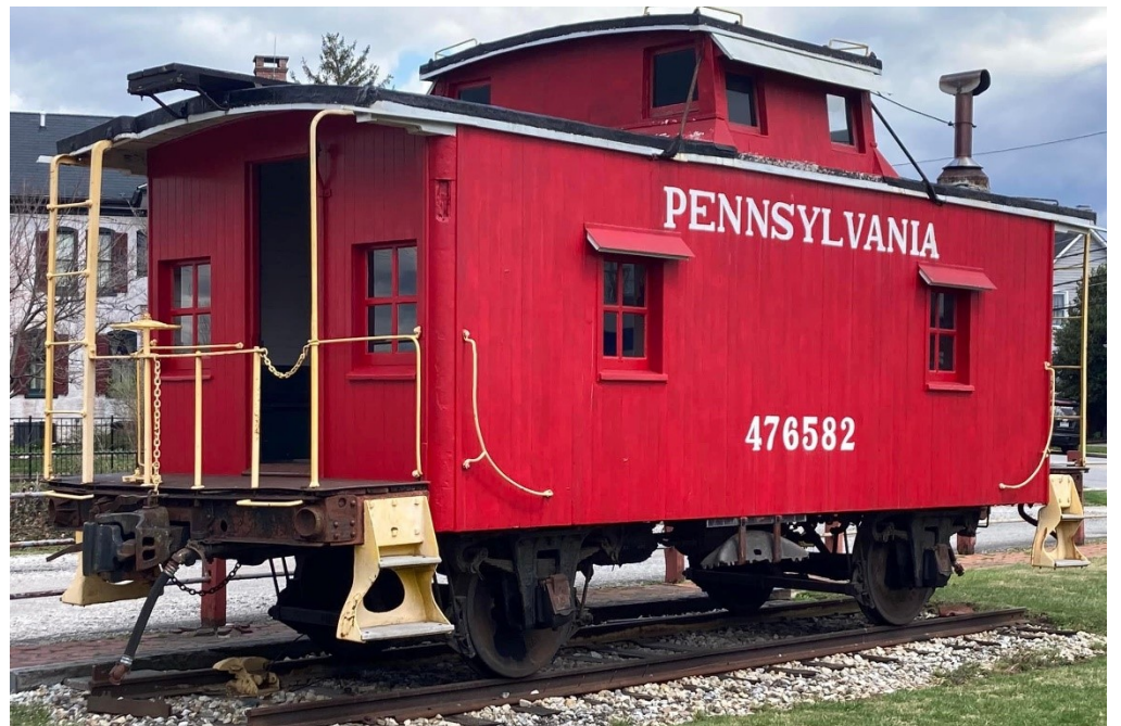
restored PRR bobber caboose #476582 parked on the grounds of the New Oxford Station
