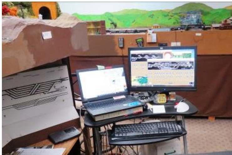
The retired DC control panel is seen on the left and the JMRI CTC panels are pictured on the laptops on the right.
