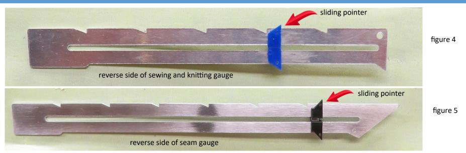
I have used the gauge to mark parallel lines on masking tape before cutting the narrow tape strips for various masking jobs (figures 6 and 7). I also find the gauge very useful for determining clearances during the conversion of a DC engine to DCC. Using the movable pointer as a depth gauge I can determine whether there will be enough clearance for the new decoder between the engine shell and the chassis/motor structure (figures 8 and 9 on next page).
