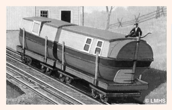
Since transport was accomplished by connecting systems of railroads and canals, the boats were constructed in sections. They could be coupled together when afloat and disconnected and placed on suitably designed eight wheeled cars for transport over the railroad. In this way, freight was carried over the entire systems without transferring from cars to boats, or vice versa.
