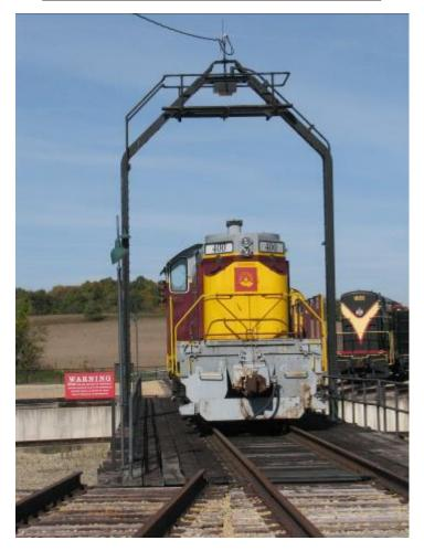
ALCO T6 #400 sits on the turntable at the Age of Steam Roundhouse complex in Sugarcreek, OH. Built in 1968, this 1,000 HP transfer engine possessed higher speeds and greater speed transitioning than an ordinary switcher. These characteristics enabled it to "transfer" freight cars between freight yards.
