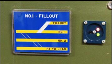
An example of the fascia-mounted turnout controllers and the accompanying track diagram. The color of the LEDs shows the position of the switch, and the diagram (which is inside a baseball card sleeve) indicates the switch associated with the controller.
