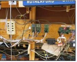
A view of more of the electronics on the layout. These boards drive block occupancy, the servos that control turnouts, and the signals around the railroad. All of this hardware is connected to a computer and controlled via JMRI (Java Model Railroad Interface).
