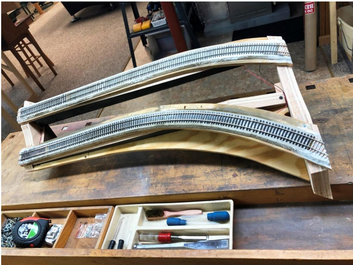
The liftout has wedges on each end which nest perfectly into V-blocks secured to the layout benchwork; thus assuring consistent alignment of the liftout tracks with the approach tracks. The wedges and V-blocks were band sawed from rectangular pieces of wood 1.75" thick. One piece is the V-block and the other is the wedge.
