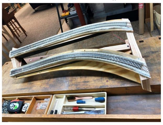
The liftout has wedges on each end which nest perfectly into V-blocks secured to the layout benchwork; thus assuring consistent alignment of the liftout tracks with the approach tracks. The wedges and V-blocks were band sawed from rectangular pieces of wood 1.75" thick. One piece is the V-block and the other is the wedge.
