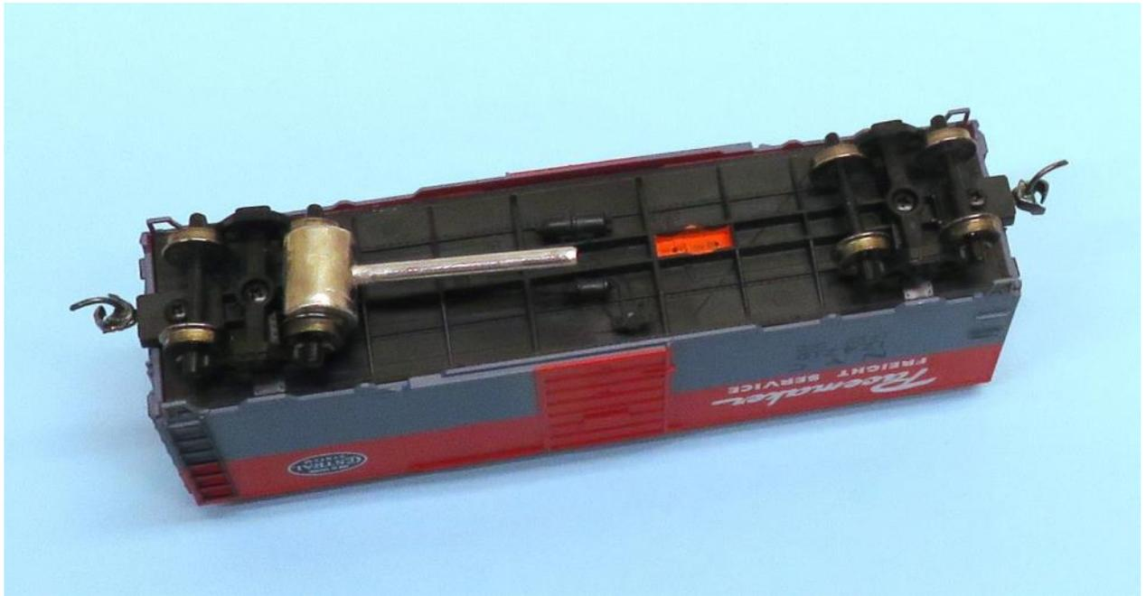
If the wheel gauge indicates too narrow a wheel spacing (gauge will not fit snugly between inside wheel backs) or too large a wheel spacing (gauge will rock between wheel backs), the wheels will need adjustment. This task can be accomplished by twisting and moving the wheels with your left and right fingers, increasing or decreasing the distance. The correction can then be verified by applying the wheel gauge. This procedure may be repeated as necessary.
