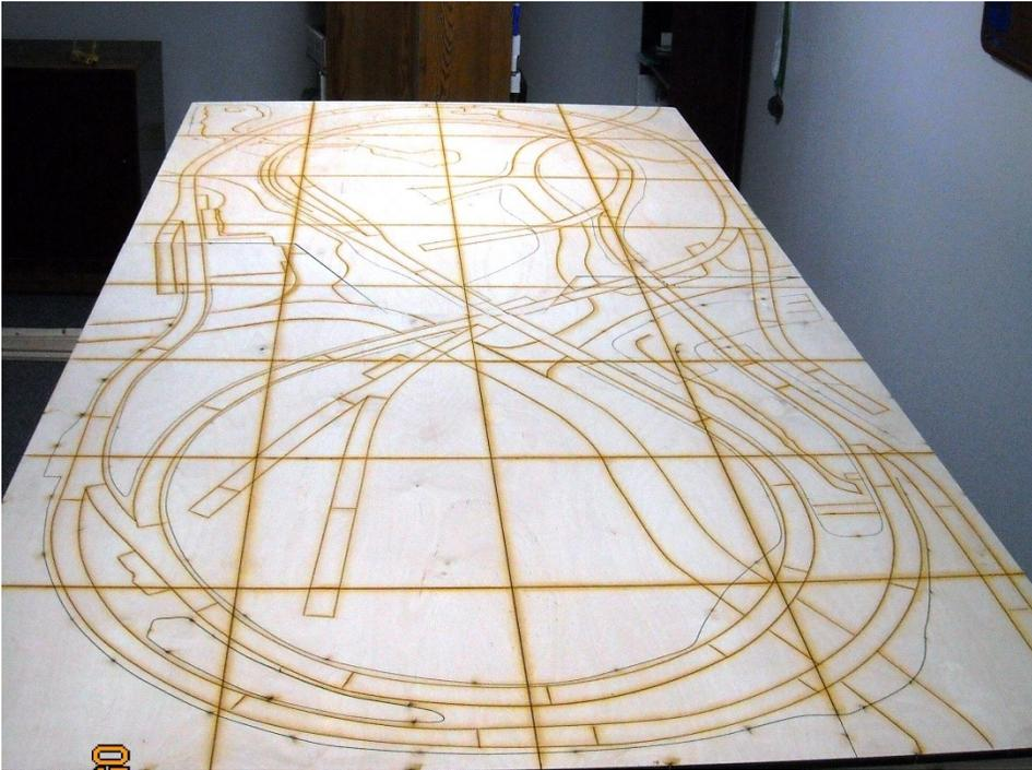
The elevated sections of the track plan were cut through the plywood using a laser. The cuts allowed the elevated portions to be raised from the base elevation.
