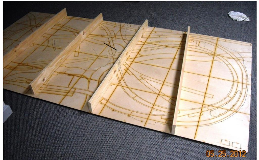
laser printed track plan added to plywood
