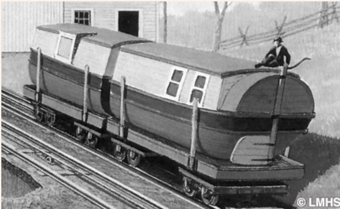
*Since transport was accomplished by connecting systems of railroads and canals, the boats were constructed in sections. They could be coupled together when afloat and disconnected and placed on suitably designed eight wheeled cars for transport over the railroad. In this way, freight was carried over the entire systems without transferring from cars to boats, or vice versa.*
