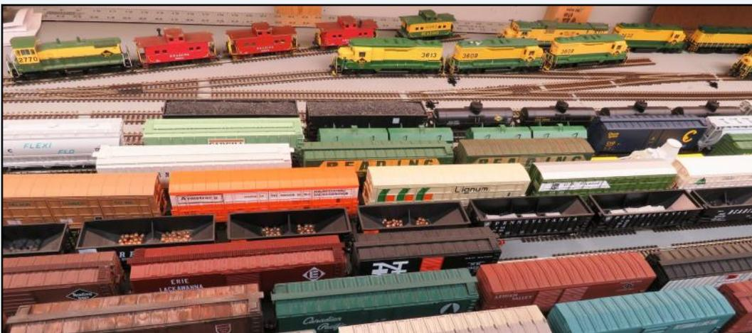
Another view of Reading Yard. Tom has between 300-400 cars on the rail-road from many different manufacturers, but has yet to weather many of them. All cars have Kadee couplers and resistors on the axles to support occupancy detection, and are weighted to NMRA standards before being put into service.
