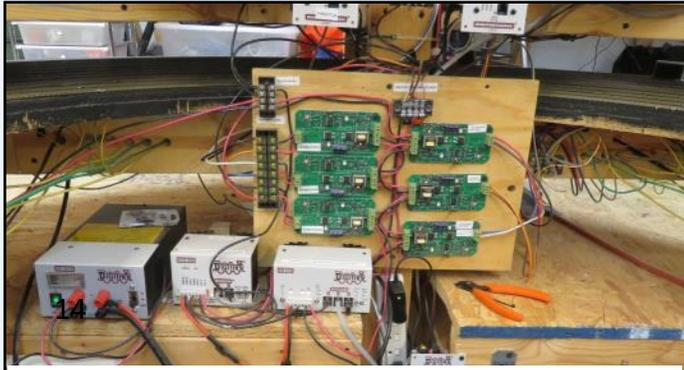
A view of the Digitrax power supply, command station and PSX circuit breaker in the center aisle of the layout. Additional boosters and circuit breakers are installed around the layout for power and short management.
