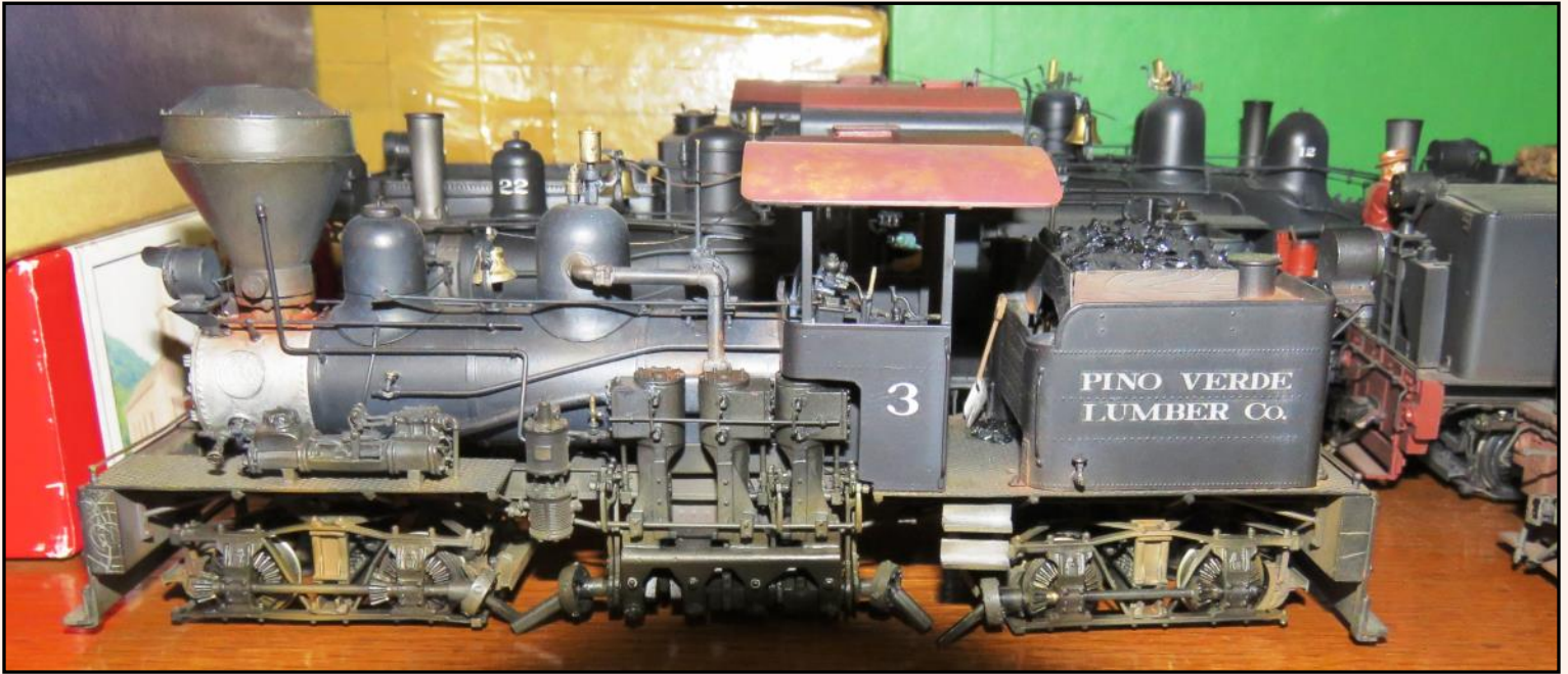
This On3 Shay locomotive was built for Tom by a Japanese modeler who became a close friend early in Tom's career. It is a highly detailed Kemptron kit with a rare left-sided steam piston driving assembly.
