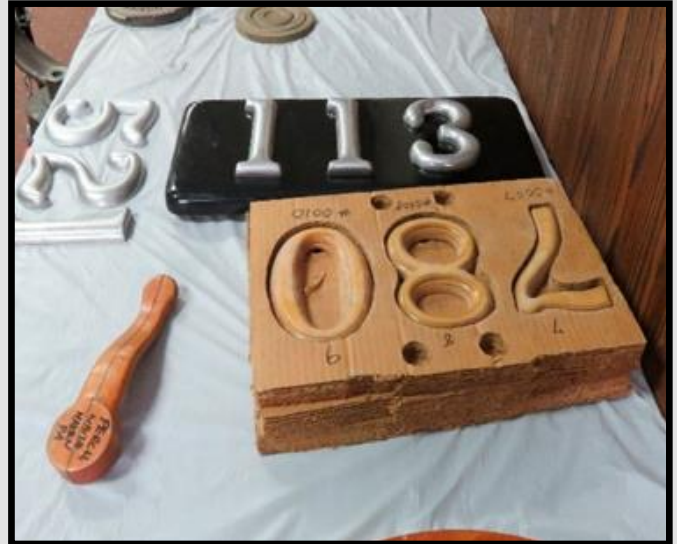
Bernie's wooden patterns used for casting engine number and bell cradle crack arm— Rich Wurst photo
