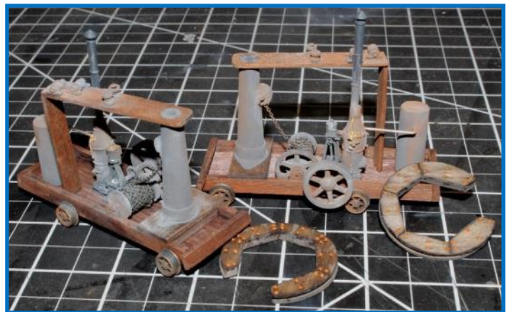
Swing gear chain sheaves installed on wooden support structure.
